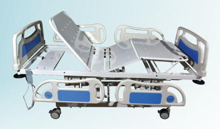
The C.R. sheet top is uniformly perforated in four sections with two electrical motors for back rest and height adjustment, two screw mechanism for trendelenburg, reverse trendelenburg and knee rest. Detachable ABS bows, IV stand and ABS railings. The entire structure is mounted on 125mm dia castor wheels – two with brake. Pretreated and powder coated.
